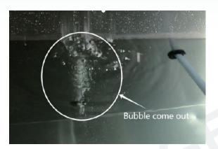
(5) Keep injecting water DIRECTLY into the tub water inlet until no more bubbles are coming out from the water outlet. This may take 2-3 minutes. When done, please remove the hose.
