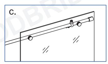
5. Loose the screws on the Glass Bracket (16), align the hole of the Glass Bracket to the holes on the Stationary Glass (14). Secure the Upper Guide Rail (4) to the Stationary Glass by fastening the screws on the Glass Bracket.
