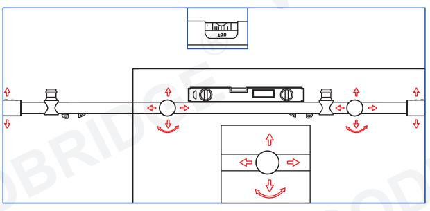
Adjust the location of the Guide Rail Brackets, mark down the location of the Stationary Glass.
