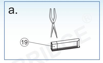
20. Place the black Gasket Cap (19) into the hole of the Guide Rail (4). Place the Hole Filler (20) into the hole of the Guide Rail (4).
