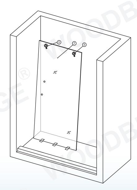
Attention: Need to loose the small allen screws before loosing the long allen screw on the roller
