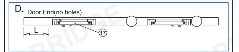
2. Your Upper Guide Rail (4) has been precut for your Shower model opening width: 48" or 60" for shower width. If W-width of your wall-to-wall opening is equal to the size of your shower model, it is unnecessary to cut the Upper Guide Rail and you can continue to Step 3. If W-width of your wall-to-wall opening is less than the size of your Shower model, you will need to cut the Upper Guide Rail from the end which is farther from the Glass brackets (16) holes.
