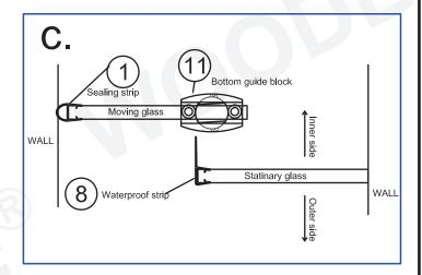
17. Attach the Side Anti-Water Strip (8) to the edge of the Stationary Glass (14) and the Bumper Strip to the Glass Door(7). Use a razor knife to trim the Side Anti-Water Strip(8) at the top to avoid interfering with the Upper Guide Rail(4).
