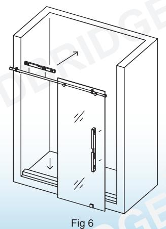
6. Place the Stationary Glass Assembly against the wall. Make sure the Stationary Glass and the Upper Guide Rail (4) are leveled.
