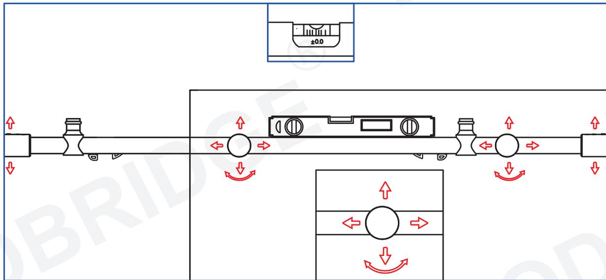
Adjust the location of the Guide Rail Brackets, mark down the location of the Stationary Glass.
