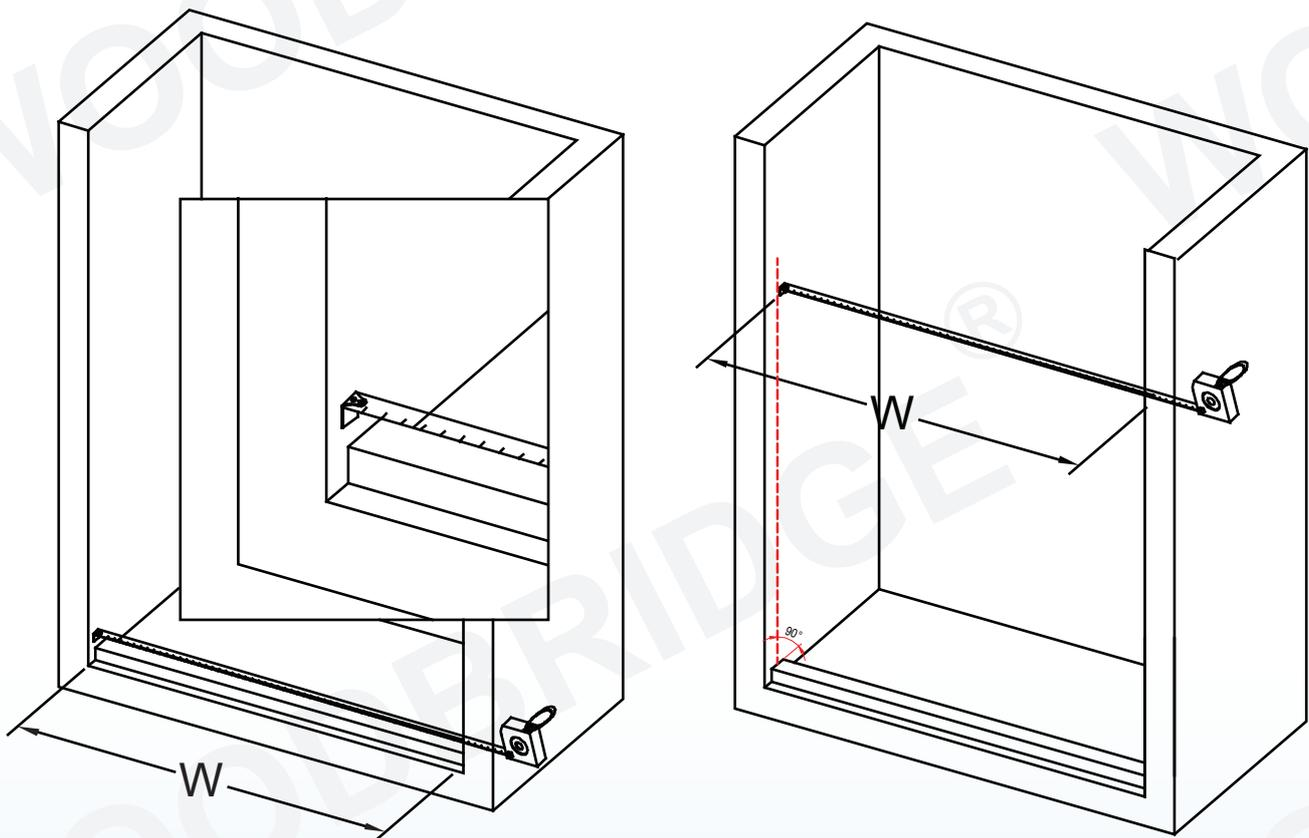
1. Measure the distance between two finished walls. This distance is marked as W.
