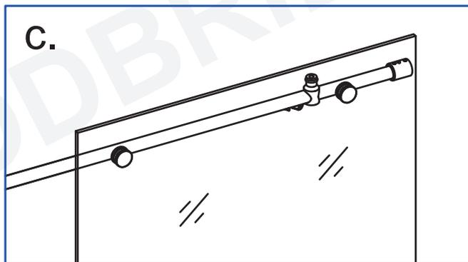
5. Loosen the screws on the Glass Bracket (16), align the hole of the Glass Bracket to the holes on the Stationary Glass (14). Secure the Upper Guide Rail (4) to the Stationary Glass by fastening the screws on the Glass Bracket.
