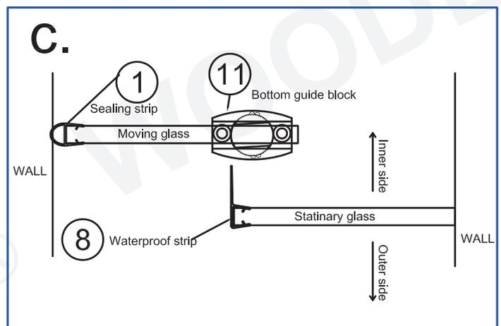
17. Attach the Side Anti-Water Strip (8) to the edge of the Stationary Glass (14) and the Bumper Strip to the Glass Door (7). Use a razor knife to trim the Side Anti-Water Strip (8) at the top to avoid interfering with the Upper Guide Rail (4). Install the handle (6) to the Glass Door (7), make sure that clear gasket and busher will be between the glass and the metal parts of the handle.
