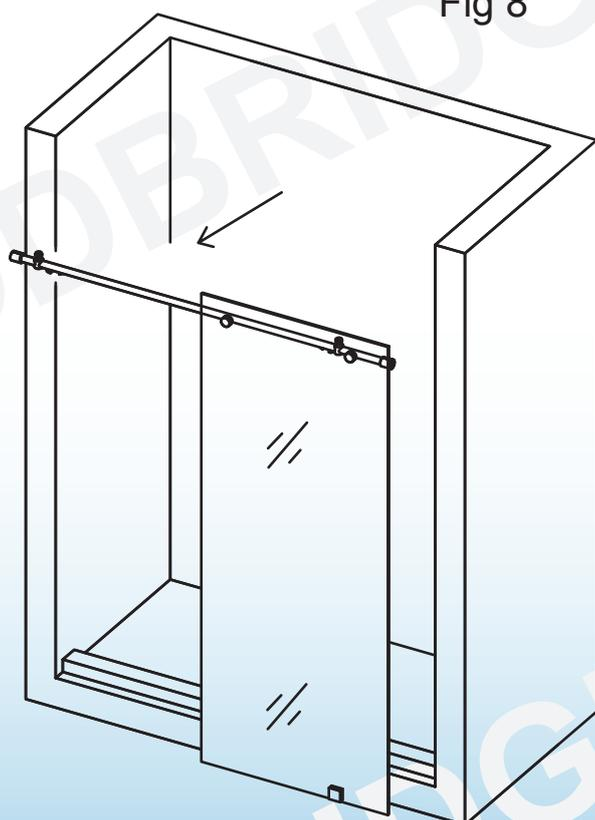
8. Drill the holes to the wall per the predrilled position using 8mm(5/16") drill bit and apply silicone into the holes, insert the Wall Anchors (12). Mount the Wall Bracket of the Guide Rail Bracket (2) to the wall by using the Screws M5×60 (15).
