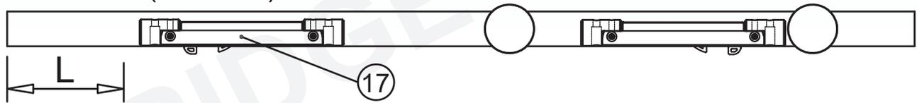
2. Your Upper Guide Rail (4) has been pre-cut for your Shower model opening width: 48" or 60" for shower width. If W-width of your wall-to-wall opening is equal to the size of your shower model, it is unnecessary to cut the Upper Guide Rail and you can continue to Step 3. If W-width of your wall-to-wall opening is less than the size of your Shower model, you will need to cut the Upper Guide Rail from the end which is farther from the Glass brackets (16) holes.
