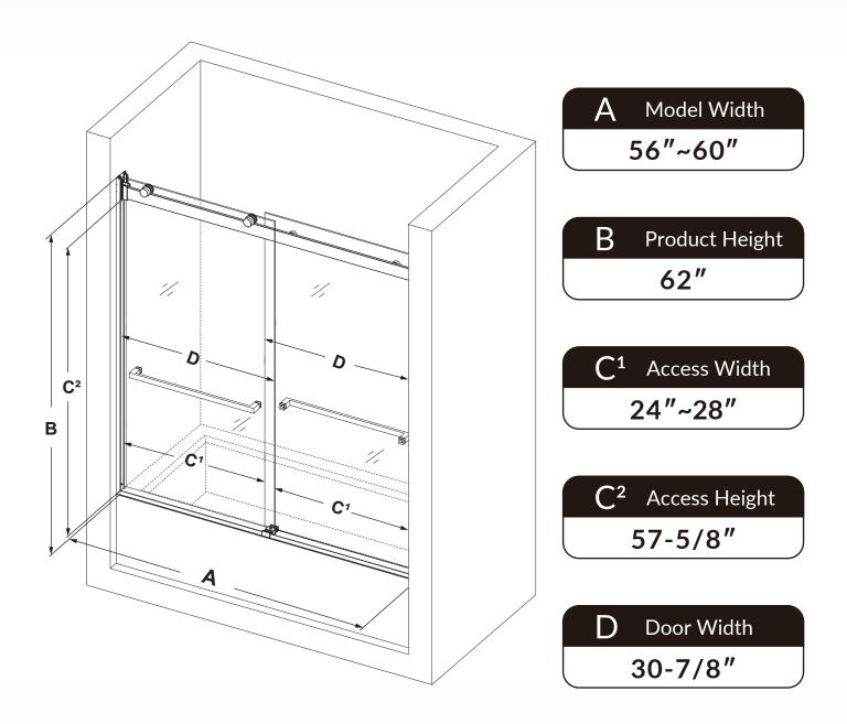
Glass Thickness: **5/16"(8mm)** Minimum Threshold Required: **3"**
