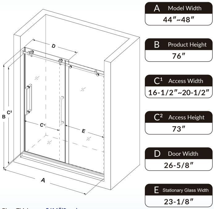
Glass Thickness: **5/16"(8mm)** Minimum Threshold Required: **3"**
