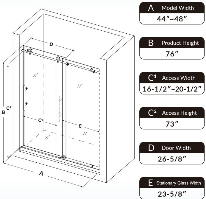
Glass Thickness: **3/8"(10mm)** Minimum Threshold Required: **2-3/4"**
