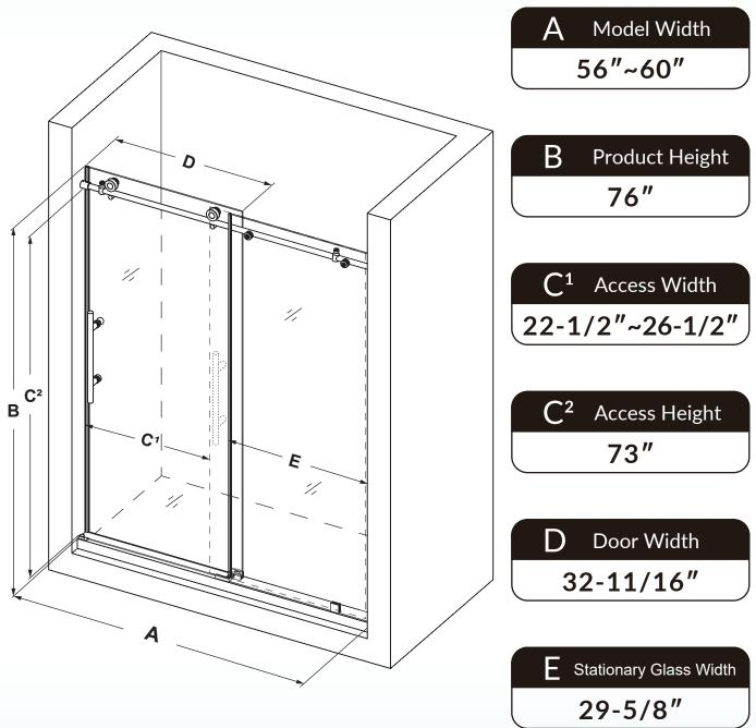
Glass Thickness: **3/8"(10mm)** Minimum Threshold Required: **2-3/4"**
