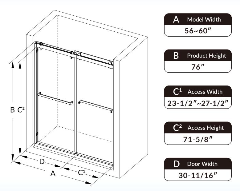
Glass Thickness: **3/8"(10mm)** Minimum Threshold Required: **3"**
