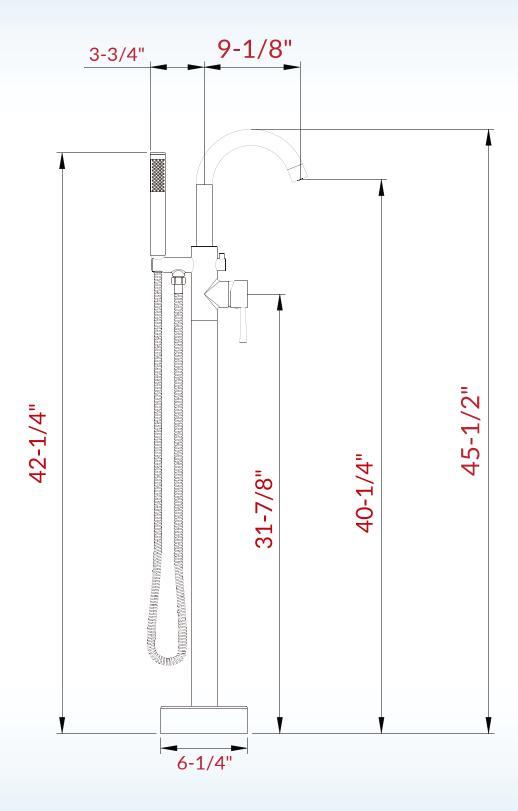
**ATTENTION!** Dimensions may vary by up to 3/8". It is highly recommended to pull all dimensions of actual model for installation and measuring purposes.
