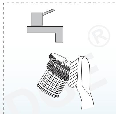
4. Clean out the filter net under running water using a toothbrush
