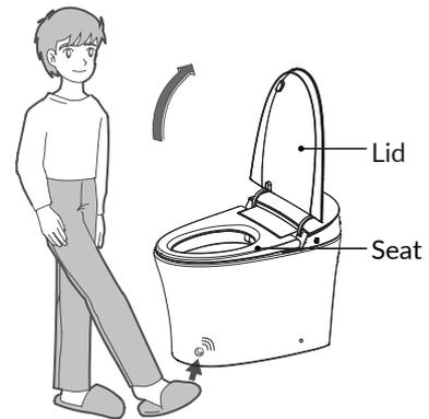
2. When the lid is open and seat closed, touch the sensing area with foot to open the seat.
