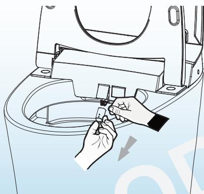
3. Use only a soft cloth or soft brush to clean. Do not pull or push the wand, to avoid damage.
