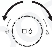
1. When seated, turn the knob clockwise to activate the front washing function, and turn it counterclockwise to activate the rear washing function. Both the rear and front washing functions will automatically transition to the drying function once completed. (Note: The default settings for water pressure, water temperature, air temperature, seat temperature, and wand position are intermediate.)
