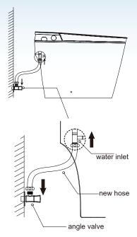
Connect the water inlet and angle valve of the toilet with the matching hose and tighten it
